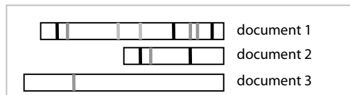
Figure 4. Display showing the location and prominence of search queries in a document.
